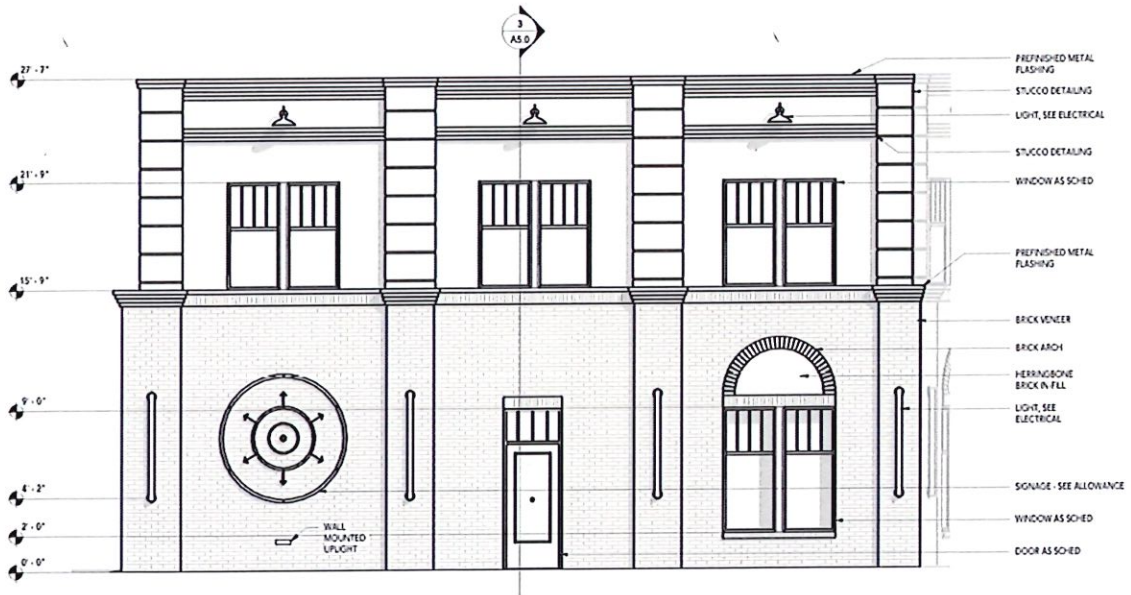
2 EXTERIOR ELEVATION - NEW WORK SCALE: 1/4" = 1'-0"
