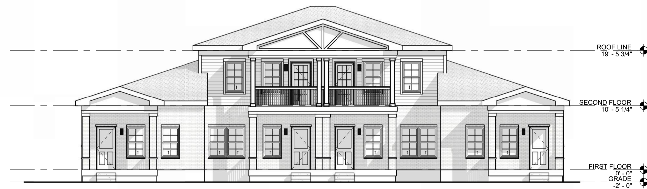
BUILDING A ELEVATION - SOUTH
